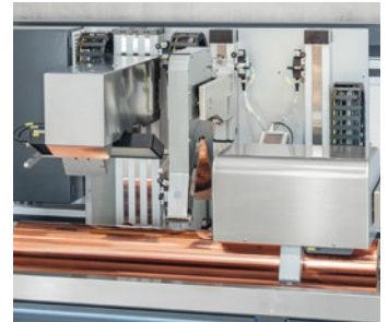
Automated measurement of diameter, roughness and engravability of the copper cylinder.
