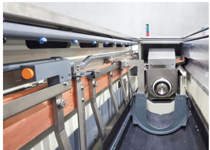
Insoluble anode with autonomous current shields
