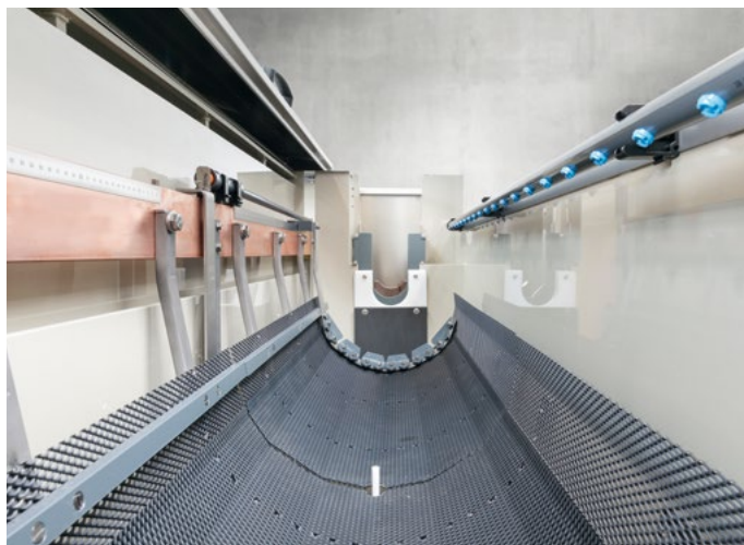
EconoLine copper tank: Insoluble anode with current shields EconoLine Kupferbad: unlösliche Anode mit Stromblende
